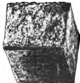
FIG. 55.—FRACTURE AT LOW TEMPERATURE.
